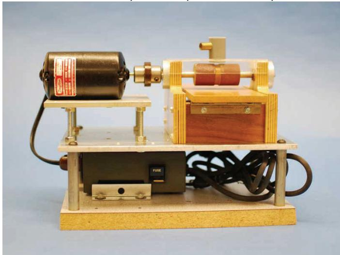
motor is similar to the one used on a "Dremel" table saw and is run with a "Dremel" speed control, which is rated for 110V, 5AMP motors. The speed control is attached to the base using Velcro, so it can be easily removed for other uses.
