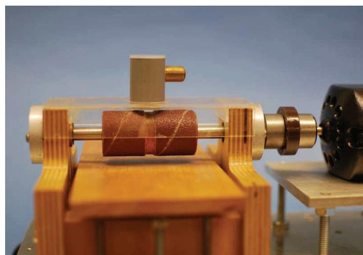
the sanding drums on the tool - paper was removed from the store-bought sleeves and re-glued onto the tool's drum.
