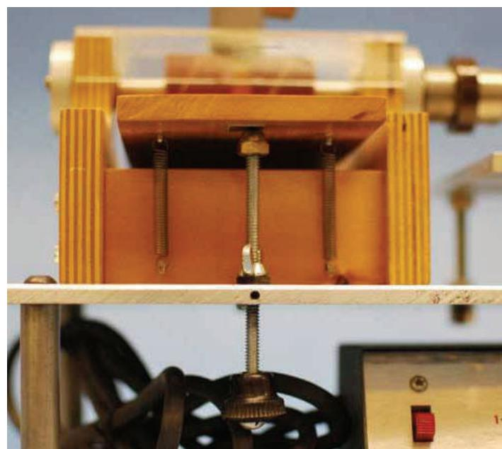
The pivoting table under the sanding drums is adjusted for desired thickness by turning the elevating nut on the support base. Springs return the table, when the adjustment is reversed. The key to doing exacting work is the flatness of the drums and adjustable table. The use of particle board or laminate is recommended. The frame base is made of Baltic Ply, and the sanding table is mounted using a piano hinge.
