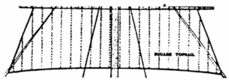
Square topsail of the GJØA from plans
